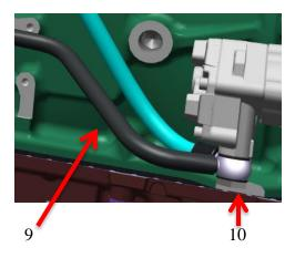
Connect part 9 into the engine using part 10 (hollow screw)
