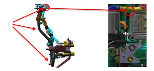
Run part 1 (fuel pipe) upwards towards the top of the engine to part 34 (radiator), and secure part 2 (hollow screw) into the hole in the tip of the upper prong of part 34 (radiator). Secure each clamp (part 7) into the predrilled holes in the engine with flange screws (part 8).
