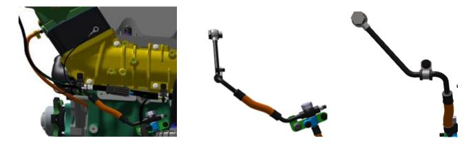
Part 24 should align with the hole in the engine block where it is supposed to mount. Mount part 24 into the engine block using part 10 (hollow screw).
