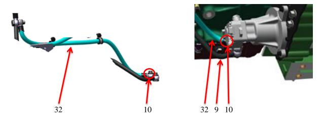
Screw the head of fuel hose part 32 into the engine block next to where fuel hose part 9 is mounted into the engine block using a hollow screw (part 10). Secure each clamp (part 7) into the predrilled holes in the engine with flange screws (part 8).
