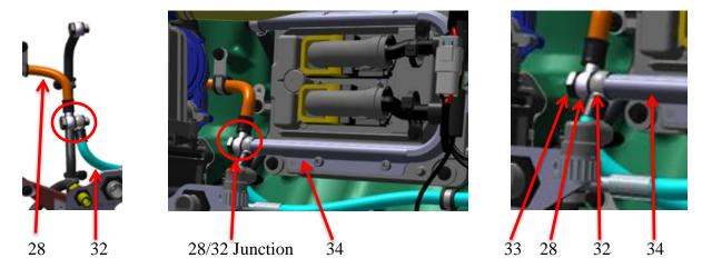
Align the opposite tip of piece 32 with the end of part 28 (fuel hose) and with the bottom rail of part 34 (radiator). Drive part 33 (hollow screw) through the heads of part 28 (fuel hose) and 32 and screw it into the tip of the lower rail of part 34 (radiator). Use both pieces of part 3 (sealing ring) as washers between pieces 33, 28, and 32.
