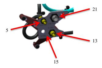
Each of the legs of part 15 (bracket) should be screwed into the engine block using the three pieces of part 17 (flange screw). With part 15 (bracket) mounted, we can begin running hoses to the correct locations.
