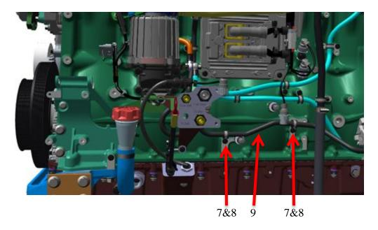
Run part 9 (fuel pipe) along the engine, and secure each clamp (part 7) into the predrilled holes in the engine with flange screws (part 8).
